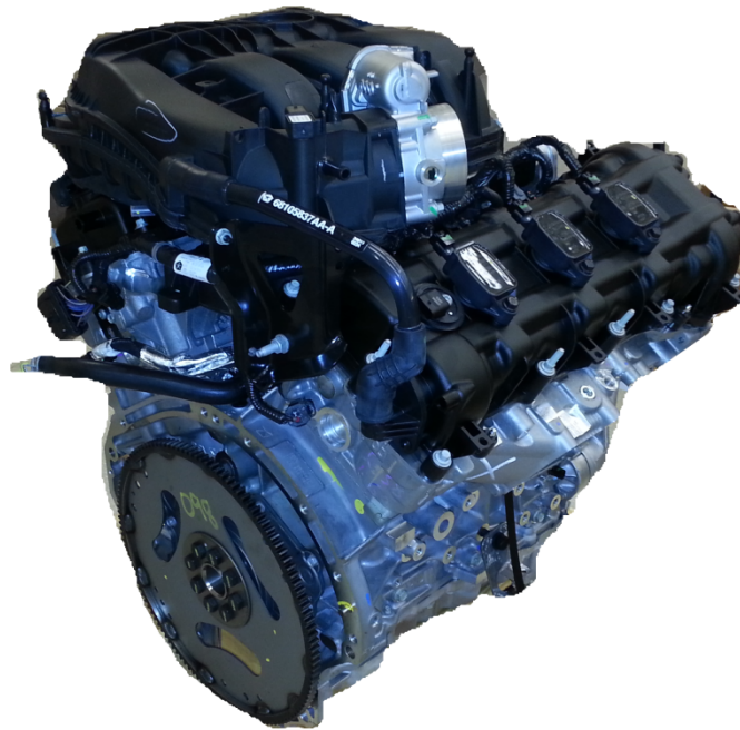
Figure 2.1 Flexplate attached to V6 3.6L engine selected for modeling and controls
